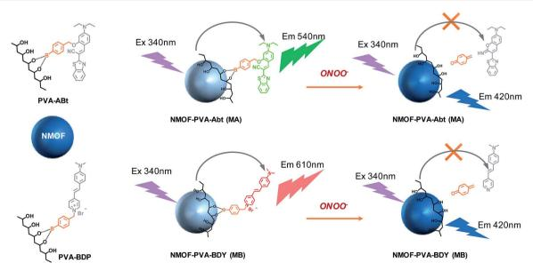
Scheme 1 Schematic of the proposed sensing mechanism of NMOF sensors.
