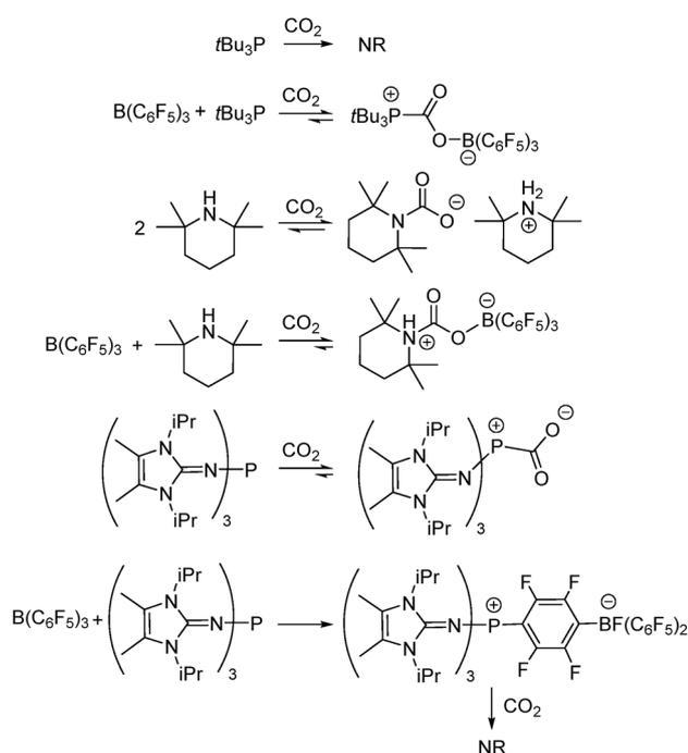
Scheme 1 Reactions of Lewis acid–base combinations with CO<sub>2</sub>. NR = no reaction.
