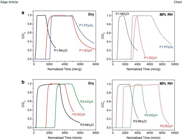
Fig. 3 Ammonia breakthrough curves for (a) P1 and (b) P2 polymers under dry (left, solid lines) and humid (right, dashed lines) conditions at 293 K. The challenge concentration ( $C_0$ ) of ammonia in air was 2000 mg m<sup>-3</sup> with a flow rate of 20 mL min<sup>-1</sup>. Once saturation was achieved, desorption curves were obtained upon purging the column with air under the corresponding initial dry or humid condition.
