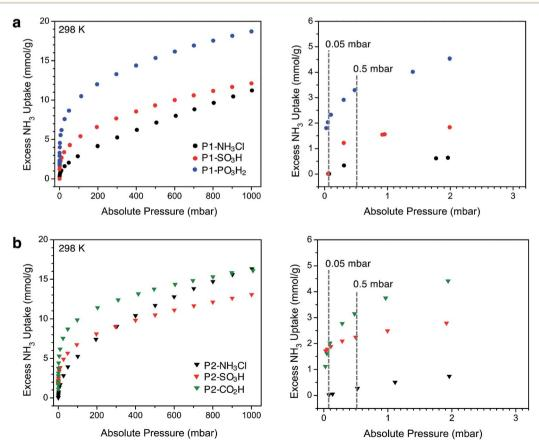
Fig. 2 Left panels: NH<sub>3</sub> adsorption isotherms for (a) P1 (circles) and (b) P2 (triangles) polymers measured at 298 K. Right panels: Low-pressure region for these plots, up to 3 mbar. Dotted gray lines are guides to compare the uptake values at 0.05 mbar (50 ppm) and 0.5 mbar (500 ppm).
