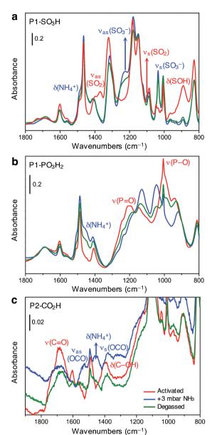
Fig. 4 Infrared spectra of (a) P1-SO $_3$ H, (b) P1-PO $_3$ H $_2$ , and (c) P2-CO $_2$ H in the 1800–800 cm $^{-1}$  spectral range collected at 298 K after its thermal activation under vacuum (red lines), equilibration with ammonia at an equilibrium pressure of 3 mbar (blue lines), and subsequent evacuation under vacuum (green lines).
