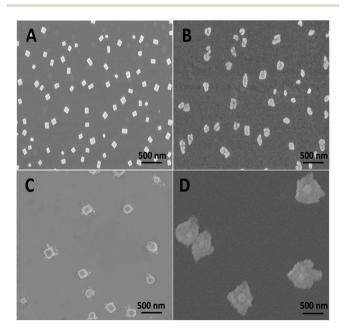
Fig. 3 Morphology characterization of PGHNs and PGHNs-DNAs by using SEM and the time effect on the co-assembly of PGHNs-DNAs. (A) Representative SEM image of PGHNs. (B-D) Co-assembly of pGalsGFP and PGHNs. These two components were mixed for indicated time, 4 h (B), 6 h (C), and 10 h (D). The average size of the nanostructures was approximately 90, 130, 200, and 500 nm, respectively.
