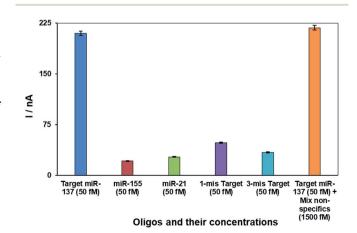
Fig. 3 Bar chart representing the specificity of the nanobiosensor in different ratios of the target miR-137 *versus* one-base mismatched target, three-base mismatch target and non-specific target (based on four replicates).
