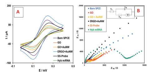
Fig. 2 Electrochemical analysis of the different stages of nanobiosensor preparation using (A) CV, and (B) EIS analysis in  $[Fe(CN)_{6}]^{3-/4-}$  solution.
