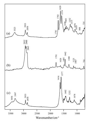
Fig. 1 (a) FTIR and (b) FT-Raman spectra of poly(hexamethylene citramide imide); (c) FTIR spectrum of the hydrolyzed polymer.
