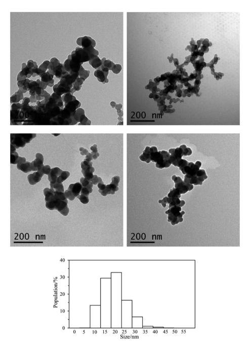
Fig. 6 TEM image of poly(hexamethylene citramide) nanoparticles formed under different pH conditions (top left, pH = 5.5; top right, pH = 7.0; bottom left, pH 9.0) and in pure water (bottom right), and the corresponding particle size distribution in pure water.
