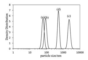
Fig. 4 DLS profiles of poly(hexamethylene citramide) particles in (a) pH = 5.5 buffer; (b) pure water; (c) pH = 6.5 buffer; (d) pH = 8.5 buffer.
