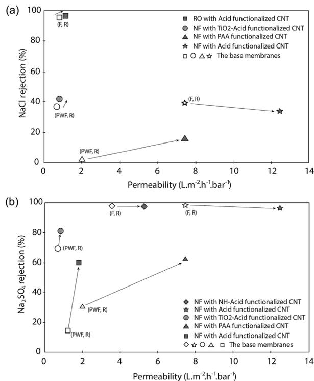
Fig. 9 Permeability vs. rejection of a functionalized CNT membrane. (a) NaCl rejection and (b) Na<sub>2</sub>SO<sub>4</sub> rejection (data from ref. 69, 73, 76, 83, 87 and 88; F: permeability of salt solution; PWF: permeability of pure water; R: salt rejection).
