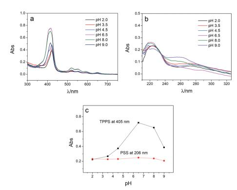
Fig. 3 DRUV spectra of PAN-[PAH/(PSS-TPPS)] $_6$  membranes prepared from PAH solutions at pH 6.5 and PSS-TPPS solutions at different pH values (a, TPPS; b, PSS), and absorbance at 405 and 206 nm at different pH values of PSS (c).
