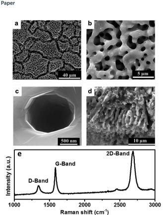
Fig. 2 (a–c) Scanning electron micrographs of the surface of graphene covered 3D stainless steel substrates at various magnifications; (d) cross-sectional image of the sample, depicting the 3D architecture until a depth of  $\sim\!10~\mu m$  from the surface; (e) Raman spectrum of the substrate, confirming 2–3 layered graphene.
