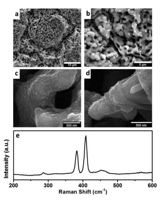
Fig. 3 (a–c) Scanning electron micrographs of MoS<sub>2</sub> covered 3D stainless steel-graphene structures. A highly conformal coating on the surface is achieved by electrodeposition technique. The porous nature of the current collector is preserved with no clogging or large particulates; (d) an isolated defect in the electrodeposition, shown to highlight the thickness of the MoS<sub>2</sub> layer; (e) Raman spectrum of the structure wherein the bands correspond to MoS<sub>2</sub>.
