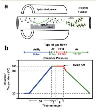
Fig. 1 (a) Schematic depiction of the CVD process for etching the surface of stainless steel while simultaneously forming graphene; (b) process conditions employed for the synthesis.
