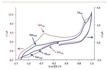
Fig. 3 CV of 5, on Pt disc electrode, in DMF containing 0.1 M Bu<sub>4</sub>NPF<sub>6</sub>, at a scan rate of  $0.1 \, \mathrm{V \, s^{-1}}$ , at a concentration of  $10^{-3} \, \mathrm{mol \, L^{-1}}$  (solid blue line) and at  $4 \times 10^{-3}$  mol L<sup>-1</sup> (aggregation, dashed red line).
