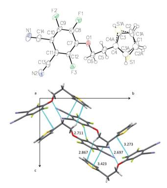
Fig. 5 X-ray crystal structure of 1a: ORTEP representation (30% probability level) (top) and projection on the (b, c) plane (bottom). The shortest intermolecular distances are indicated (in Å).
