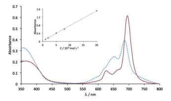
Fig. 4 UV-visible absorption spectra of 5 in chloronaphthalene (solid red line) and in dimethylformamide (dotted blue line), both at 8  $\times$  $10^{-6}$  mol L<sup>-1</sup>. The inset shows the variation of the absorbance at the maximum wavelength as a function of the concentration, in chloronaphthalene
