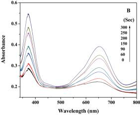
Fig. 5 (A) Typical absorbance curves of different reaction systems for 3 min in HAC–NaAc (pH = 3.8) buffer: (a) PDI–CuO +  $H_2O_2$  + TMB; (b) CuO +  $H_2O_2$  + TMB; (c) PDI–CuO + TMB; (d)  $H_2O_2$  + TMB; (e) TMB, respectively. (B) Time-dependency of peroxidase-like activity of PDI–CuO nanocomposites. The absorbance of the reaction system (TMB: 2 mM;  $H_2O_2$ : 0.25 M; PDI–CuO: 0.3 mg mL $^{-1}$ ) was monitored in time scan mode. The inset is the corresponding colorimetric photograph.
