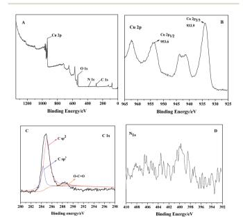
Fig. 4  $\,$  XPS spectra of PDI–CuO (A), Cu 2p (B), C 1s (C) and N 1s (D), respectively.
