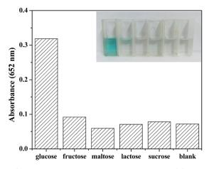
Fig. 10 Selectivity analysis for glucose detection using GOx and PDI–CuO catalyst by monitoring the relative absorbance (inset: the color change corresponding to different sample: 1.0 mM glucose, 5.0 mM fructose, 5.0 mM maltose, 5.0 mM lactose, and 5.0 mM sucrose).
