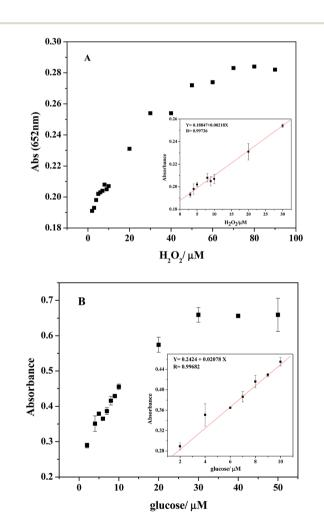
Fig. 9 (A) A dose-response curve for H<sub>2</sub>O<sub>2</sub> detection using PDI-CuO under the optimum conditions. Inset: the linear calibration plot for H<sub>2</sub>O<sub>2</sub> detection (B) A dose-response curve for glucose detection using PDI-CuO as catalysts. Inset shows the linear response of the detection system to glucose. Error bars stand for the standard deviations based on three repeated measurements.
