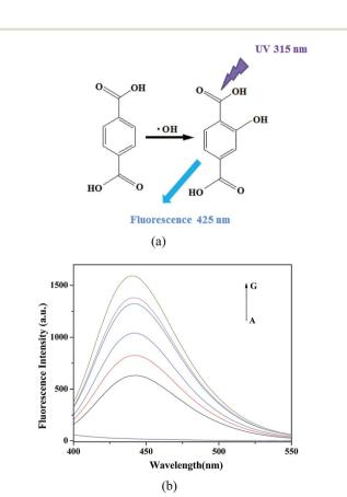
Fig. 8 (a) The reaction of TA with 'OH. (b) Fluorescent spectra of acetate buffer solution (pH = 4) containing only TA and PDI-CuO (A) or with  $H_2O_2$  (0.25 M), TA (0.5 mM) and the PDI-CuO nanocomposites with different concentration ((B) 0, (C) 20, (D) 80, (E) 200, (F) 250, (G) 300 μg mL<sup>-1</sup>) were incubated at 55 °C for 30 min. The FL excitation wavelength was fixed at 315 nm.
