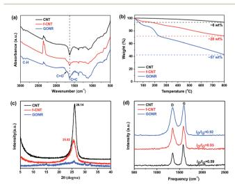
Fig. 3 Structural characterizations of pristine CNTs, f-CNTs and GONRs: (a) FTIR spectra, (b) TGA curves, (c) XRD results and (d) Raman spectra.
