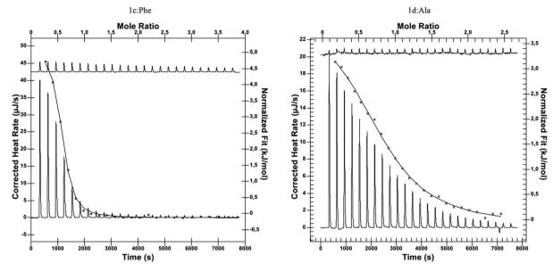
Representative thermograms of ITC experiments: L-Phe titrated to 1c (left) and L-Ala titrated to 1d (right).
