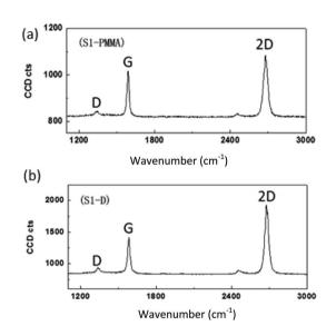
Fig. 23 Raman spectra (532 nm laser excitation wavelength) for graphene transferred onto the  ${\rm SiO_2}$ -on-Si substrate. (a) Raman spectra obtained from a sample prepared by the standard PMMA-based method. (b) Raman spectra obtained from a sample obtained by the direct transfer method. This figure has been adapted/reproduced from ref. 123 with permission from World Scientific.
