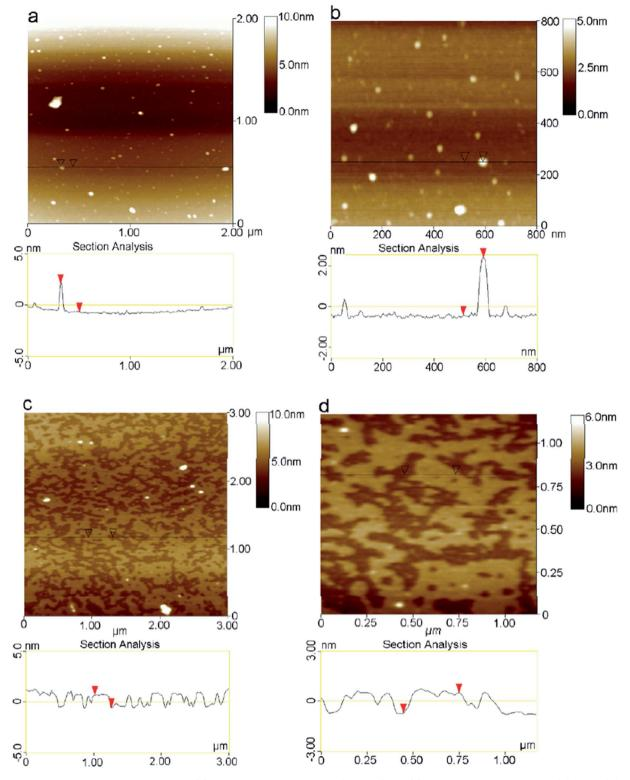
Fig. 53 Typical tapping mode AFM images of (a) few-layer graphene sheets 2  $\mu$ m  $\times$  2  $\mu$ m, (b) few-layer graphene sheets 0.8  $\mu$ m  $\times$  0.8  $\mu$ m, (c) monolayer graphene sheets 3  $\mu$ m imes 3  $\mu$ m, and (d) monolayer graphene sheets 1.25  $\mu$ m deposited on the mica substrate from dispersion, corresponding height cross-sectional profile. This figure has been adapted/reproduced from ref. 90 with permission from Elsevier.
