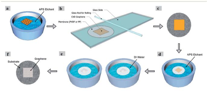
Fig. 21 Schematic of single-layer graphene transfer onto a polymeric substrate. This figure has been adapted/reproduced from ref. 117 with permission from Elsevier.
