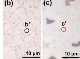
Fig. 56 (a) Low-magnification optical microscope image of as-synthesized graphene on Ni/SiO<sub>2</sub>/Si substrate using 2 sccm CH<sub>4</sub>, 30 s growth duration and a fast cooling process. (b) & (c) High-magnification images of the regions corresponding to the region in (a). Dashed circle in (a) presents a boundary where graphene is synthesized. This figure has been adapted/reproduced from ref. 179 with permission from Springer.
