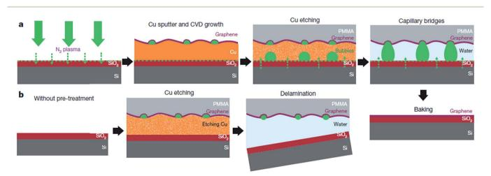
Fig. 19 Interpretation of the face-to-face technique for transferring graphene mediated by capillary bridges. (a) Schematic drawing showing the 'bubble seeding' by plasma treatment, CVD growth, Cu film etching, formation of capillary bridges and removal of water and PMMA. (b) Schematic illustration showing that in the absence of plasma treatment, delamination of the film results. This figure has been adapted/reproduced from ref. 112 with permission from Nature Publishing Group.
