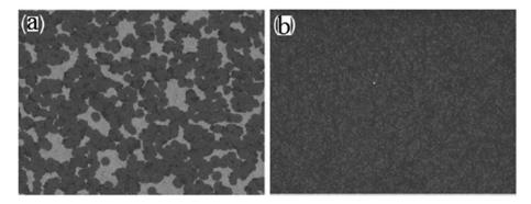
Fig. 41 (a) SEM image (12  $\mu$ m  $\times$  9  $\mu$ m) and (b) SEM image (12  $\mu$ m  $\times$  9  $\mu$ m) of a fully graphene-covered surface, showing a coherent graphene layer. This figure has been adapted/reproduced from ref. 152 with permission from Elsevier.
