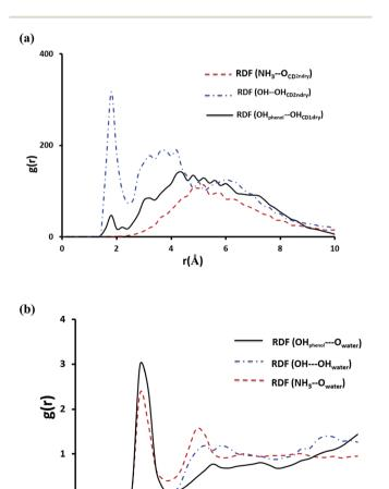
Fig. 11 The RDF of hydrogen bonding interactions for NP-βCD complex plotted as a function of separation distance r (in Å) between donor and acceptor (a) interaction of NP with host (b) interaction of NP with water. These plots were obtained from MD trajectories after equilibration of the inclusion complex.
