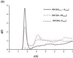
Fig. 12 The RDF of hydrogen bonding interactions for NP-CB7 complex plotted as a function of separation distance r (in Å) between donor and acceptor (a) interaction of NP with host (b) interaction of NP with water. These plots were obtained from MD trajectories after equilibration of the inclusion complex.
