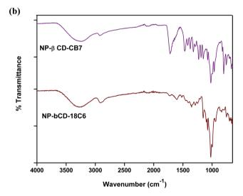
Fig. 3 FT-IR spectra of (a) binary complexes (b) ternary complexes of NP- $\beta$ CD with CB7 and 18C6.
