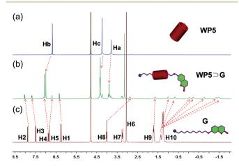
Fig. 3 Partial  $^1\text{H}$ -NMR (400 Hz, D $_2\text{O}$ , 293 K) spectra: (a) WP5 (10.0 mM); (b) WP5 (10.0 mM) and G (10.0 mM); (c) guest molecule G (10.0 mM).
