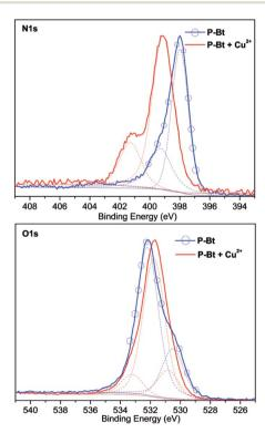
Fig. 4 XPS analysis of P-Bt and corresponding  $Cu^{2+}$  based MSP. The molar ratio between the unimer and  $Cu^{2+}$  is (1 : 1).
