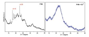
Fig. 3 X-ray diffraction pattern of P-Bt and its  $Cu^{2+}$  based MSP. The molar ratio between the unimer and  $Cu^{2+}$  is (1 : 1).
