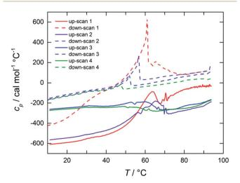
Fig. 6 Raw DSC thermograms of a 10.0 mM NaManLC sample (pH 12.0). Up-scans (solid lines) and down-scans (dashed lines) are obtained with a scan rate of 60 °C h<sup>-1</sup> on the same sample.
