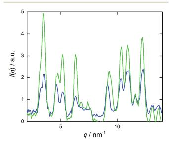
Fig. 3 WAXS patterns of crystalline (green) and sonicated (blue)  $10.0 \ \text{mM}$  NaManLC samples (pH 12.0).
