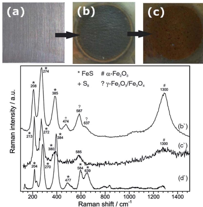
Fig. 14 Shows images of (a) bare metal before exposure to saline  $\text{H}_2\text{S}$  saturated acetic solution, (b) area of exposure after anodic polarization for 44 h at 200 mV above  $E_{\text{corr}}$ , with Raman spectrum (b'); and (c) corrosion products after aging in air for 90 d, with Raman spectrum (c'), along with the reference Raman spectrum for mackinawite (d').<sup>125</sup> Reproduced by permission of The Electrochemical Society.
