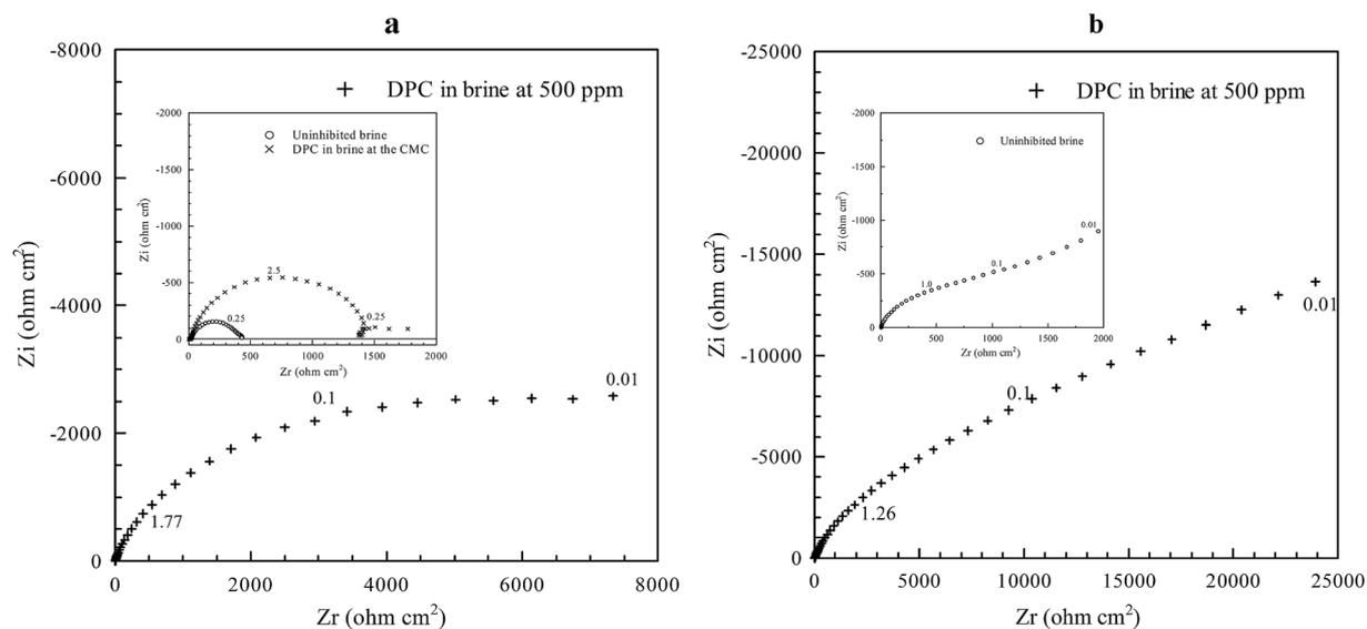
Fig. 8 Electrochemical impedance spectroscopy Nyquist plots for (a) CO<sub>2</sub>-saturated brine with 500 ppm DPC (inset: un-inhibited brine and DPC at the CMC) and (b) N<sub>2</sub>-saturated brine with 500 ppm DPC for carbon steel after 4 h immersion.<sup>83</sup> Reprinted with permission from ref. 83. Copyright 2014, American Chemical Society.
