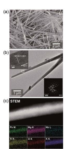
Fig. 2 (a) SEM image of PMN-PT NWs synthesized by a hydrothermal method. (b) TEM image of PMN-PT NWs. The Left-top inset is a HRTEM image of a single NW showing that lattice fringes of the (110) plane and the right-bottom image shows the SAED pattern when the electron beam is coherent along the [001] plane. (c) STEM image and EDS mapping of a PMN-PT NW.
