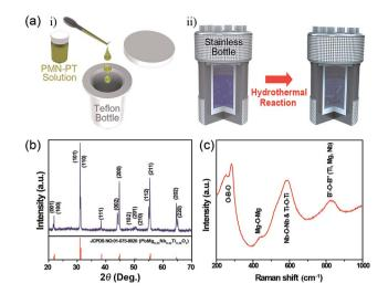
Fig. 1 (a) Schematic representation of the synthesis procedure for the preparation PMN–PT NWs by a hydrothermal method. (i) PMN–PT solution prepared by a sol–gel method used as seed. (ii) PMN–PT nuclei grown as NWs under hydrothermal conditions. (b) XRD pattern of PMN–PT NWs. (c) Raman spectrum of PMN–PT NWs.
