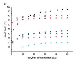
Fig. 4 Concentration dependence of the UCST-type cloud points of the polymers P-1<sub>575</sub> (+,  $\times$ ), P-3<sub>95</sub> ( $\nabla$ ,  $\nabla$ ), P-4<sub>585</sub> ( $\Diamond$ ,  $\spadesuit$ ), P-5<sub>50</sub> ( $\star$ ,  $\star$ ), P-6<sub>500</sub> ( $\bigcirc$ ,  $\bullet$ ), P-7<sub>85</sub> ( $\triangle$ ,  $\triangle$ ), and P-8<sub>100</sub> ( $\square$ ,  $\blacksquare$ ): (a) in H<sub>2</sub>O (open symbols), (b) in D<sub>2</sub>O (full symbols).
