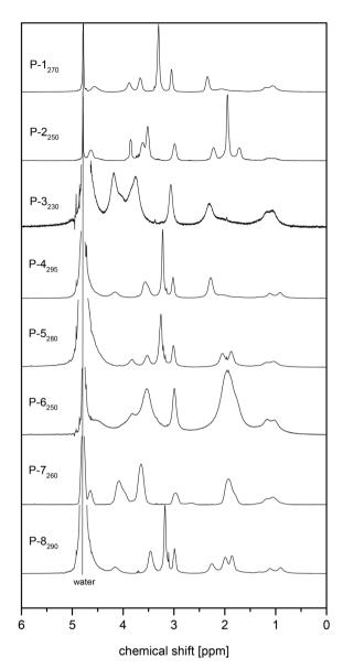
Fig. 3 <sup>1</sup>H NMR spectra of poly(sulfobetaine methacrylate)s P-1-P-8 in D<sub>2</sub>O with added NaCl (solvent signal at 4.78 ppm); from top to bottom:  $P-1_{270}$ ,  $P-2_{250}$ ,  $P-3_{230}$ ,  $P-4_{295}$ ,  $P-5_{280}$ ,  $P-6_{250}$ ,  $P-7_{260}$  and  $P-8_{290}$ .
