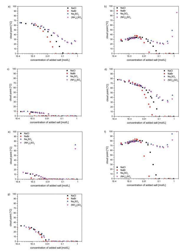
Fig. 5 Evolution of UCST-type cloud points of the polymer solutions in  $H_2O$  (50 g  $L^{-1}$ ) containing inorganic salts for (a) P-1<sub>575</sub>, (b) P-3<sub>95</sub>, (c) P-4<sub>585</sub>, (d) P-5<sub>50</sub>, (e) P-6<sub>500</sub>, (f) P-7<sub>85</sub>, and (g) P-8<sub>100</sub>. ( $\blacksquare$ ) = NaCl, ( $\blacksquare$ ) = NaBr, ( $\blacktriangle$ ) = Na<sub>2</sub>SO<sub>4</sub>, ( $\blacktriangledown$ ) = (NH<sub>4</sub>)<sub>2</sub>SO<sub>4</sub>.
