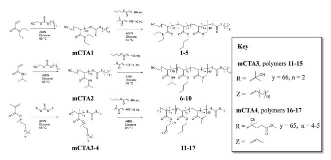
Scheme 2 Synthesis of the four corona-forming macroCTA blocks (mCTA1-4) and their subsequent chain extension to yield the amphiphilic diblock copolymers (1-17).
