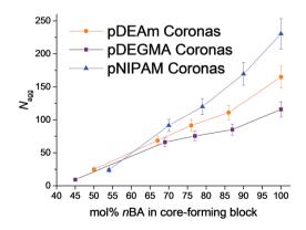
Fig. 2 Variation in the particles'  $N_{\rm agg}$  with the molar fraction of hydrophobic nBA in the core-forming block, as determined by SLS analysis. Micelles with pDEAm (polymers 1–5, orange circles), pNIPAM (polymers 6–10, blue triangles) and pDEGMA coronas (polymers 11–15, purple squares) are shown. Error bars represent 10% error.
