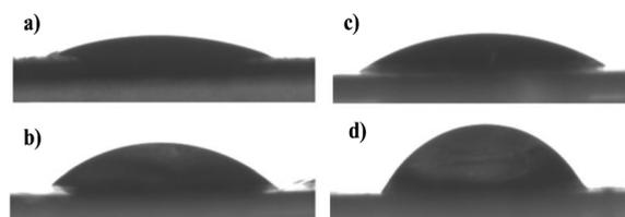
Fig. 7 Contact angles of water (a) and glycerol (b) in pure BC and water (c) and glycerol (d) in oxidized BC, respectively. Droplets of 3  $\mu\text{L}$  of water and glycerol were placed for 60 s over the BC films. (Adapted with permission from ref. 143: C. Lai, L. Sheng, S. Liao, T. Xi and Z. Zhang, Surface characterization of TEMPO-oxidized bacterial cellulose, *Surf. Interface Anal.*, 2013, **45**, 1673–1679. Copyright 2013, John Wiley & Sons, Ltd.)
