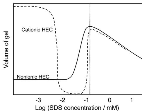
**Fig. 4** The effect of addition of an anionic surfactant (SDS) changes dramatically the volume of polymer gels as illustrated here for a nonionic polymer (HEC) and an oppositely charged polyelectrolyte (cationic HEC). (With permission from ref. 112: J. Sjöström and L. Piculell, Simple gel swelling experiments distinguish between associating and nonassociating polymer–surfactant pairs, *Langmuir*, 2001, **17**, 3836–3843. Copyright 2001, American Chemical Society.)
