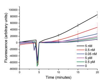
Fig. 4 Sensitivity of the biosensor. The fluorescence signal after the addition of different concentrations of  $A_0$  to a mixture of  $P_0A_1A_2$ ,  $P_1S$ , and  $P_2S$  (50 nM each) was monitored for 15 minutes in the presence of 0.1 U  $\mu L^{-1}$  of exo III at room temperature (25 °C). (At  $t = \sim 5$ , the signal dropped because the spectrofluorometer was opened when exo III was added.)
