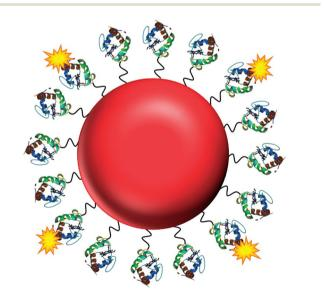
Fig. 1 The NO nanobiosensor: cytochrome c (structure obtained from the Protein Data Bank – PDB ID 1HRC)<sup>28</sup> fluorescently tagged with Alexa Fluor 488 (yellow) assembled onto a gold nanoparticle (red) surface via a SPDP linker (black).
