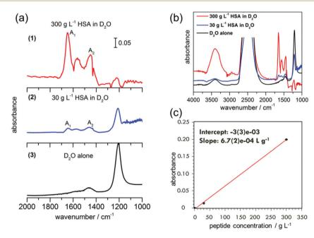
Fig. 4 (a) ATR-IR spectra of (1) HSA in  $D_2O$  (300 g  $L^{-1}$ ), (2) HSA in  $D_2O$  (30 g  $L^{-1}$ ) in 10 nm deep Ge ATR-IR nanochannel devices and (3) bulk  $D_2O$ alone obtained on the Ge ATR-IR crystal. A1 (1649 cm<sup>-1</sup>) and A2 (1450 cm<sup>-1</sup>) indicate the amide I and amide II peaks, respectively. (b) The extended spectra of the same, from 4000 to 1000 cm<sup>-1</sup>. (c) Peak absorbance of amide I mode versus concentration.
