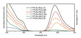
Fig. 2 Absorption (left) and PL (right) spectra of  $Mn^{2+}$ :  $ZnSe_{1-x}S_x$  NCs with varying dichalcogenide precursor ratios. The NC first absorption peak shifts from  $\sim 390$  nm for  $Ph_2Se_2$  alone (1) to a broad feature at  $\sim$  340 nm for Me<sub>2</sub>S<sub>2</sub> alone (5). The PL peak red-shifts from 586 nm to 589 nm with increasing S. For 4, very little luminescence was detected and for 5 no luminescence was detected
