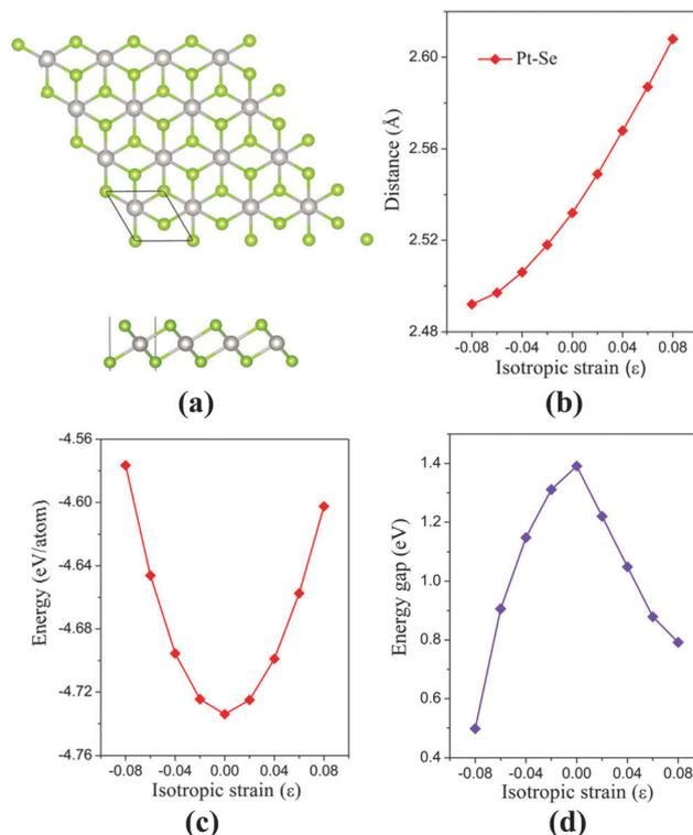
Fig. 1 (a) Top and side views of monolayer PtSe<sub>2</sub>. The green and gray balls represent Pt and Se atoms, respectively. (b) Pt–Se bond length versus isotropic in-plane strain. (c) Total energy per atom of the monolayer PtSe<sub>2</sub> versus isotropic strain. (d) Computed band gap of monolayer PtSe<sub>2</sub> versus isotropic strain.
