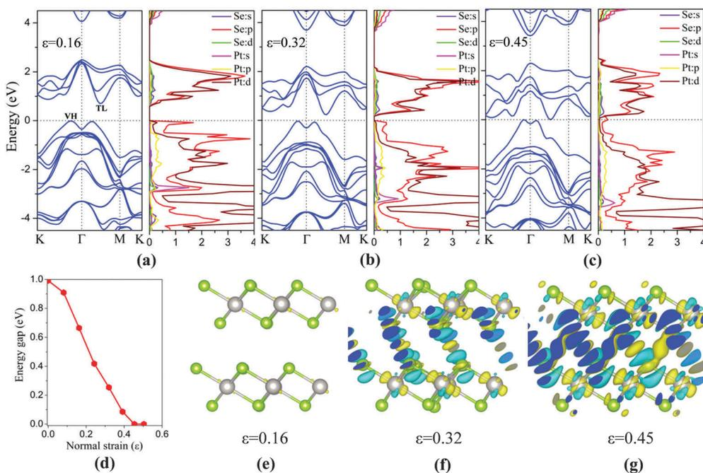
Fig. 6 (a–c) Computed band structure and partial densities of states of PtSe<sub>2</sub> bilayer under three different VCS values, with the corresponding differential charge densities plotted in (e–g). The Fermi level is located at 0 eV. (d) Band gap of bilayer versus normal strain.
