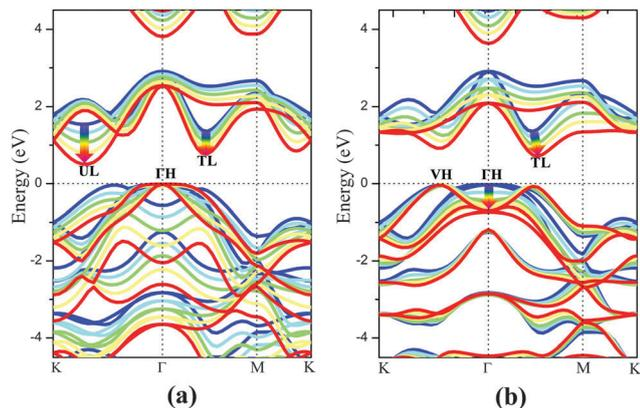
Fig. 2 Computed band structures of monolayer PtSe<sub>2</sub> under (a) isotropic compressive, and (b) isotropic tensile strain. The bands with different colors denote the band structures under different strain, *i.e.*, blue ( $\epsilon = 0\%$ ), cyan ( $\epsilon = \pm 2\%$ ), green ( $\epsilon = \pm 4\%$ ), yellow ( $\epsilon = \pm 6\%$ ) and red ( $\epsilon = \pm 8\%$ ). The Fermi level is located at 0 eV.
