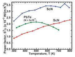
Fig. 2 Thermoelectric power factor  $S^2\sigma$  of ScN (the bottom curve shows our first data from ref. 2 and the top curve are the data of Burmistrova et al.).3 The example data for PbTe are adapted from Sootsman et al. 43
