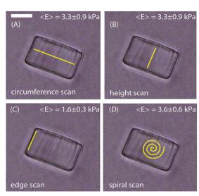
Fig. 2 Hydrogel cylinders of diameter 48  $\mu$ m and height 30  $\mu$ m were probed along the (A) circumference (B) height (C) edge and (D) in a spiral manner. The scale bar is 20  $\mu$ m.
