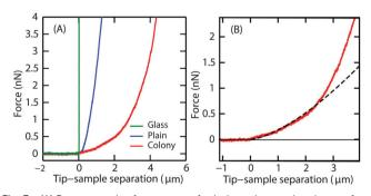
Fig. 3 (A) Representative force curves for indentation on the glass surface (green), plains of the biofilm (blue) and the superficial layer of the microcolony (red). (B) The force–indentation curve on the microcolony slowly increased up to an indentation depth of 2  $\mu m$  after which the slope of the curve increased. The force curve is fitted using the Hertz model up to a depth of 1  $\mu m$  (dashed line).
