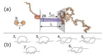
Fig. 1 (a) Schematic of Brownian dynamics simulation. A knotted polymer translocates through a pore with a force f(t) per bead. (b) Types of knots simulated (Alexander–Briggs notation<sup>46</sup>).
