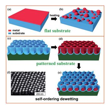
Fig. 1 Sketch illustrating dewetting of a metal film (a, b) on a flat surface and (c–e) on a patterned surface of  $TiO_2$  nanotubes (*i.e.*, template-guided dewetting); (f) SEM image of arrays of single-Auparticle-per-cavity formed by dewetting a Au film on a highly regular self-organized anodic  $TiO_2$  nanocavity layer. Fig. (f) is reproduced with permission from ref. 16.
