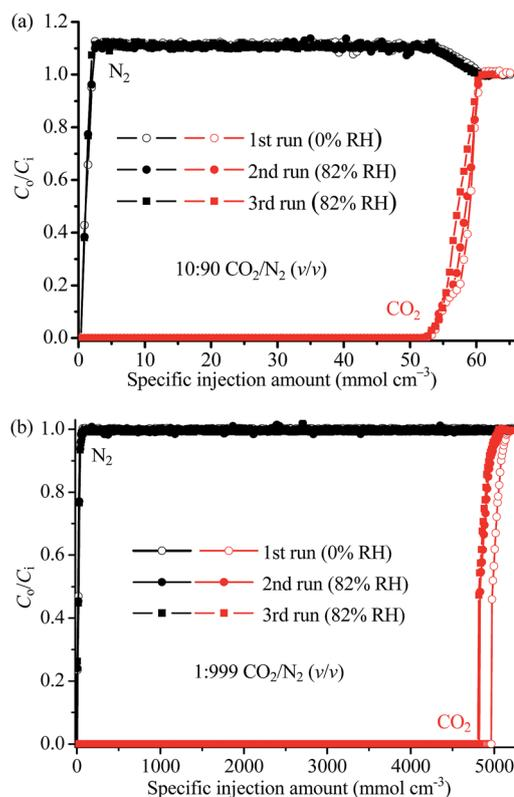
Fig. 5 Repeated breakthrough curves of the **1a** column operated at 1 bar. (a) 10 : 90 CO<sub>2</sub>/N<sub>2</sub> (v/v) at 313 K. (b) 1 : 999 CO<sub>2</sub>/N<sub>2</sub> (v/v) mixture at 298 K. Lines are drawn to guide eyes. C<sub>i</sub> and C<sub>o</sub> are the concentrations of each gas at the inlet and outlet, respectively.
