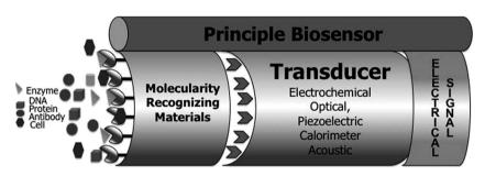
Fig. 10 Elements and components of a typical biosensor (figure by author)
