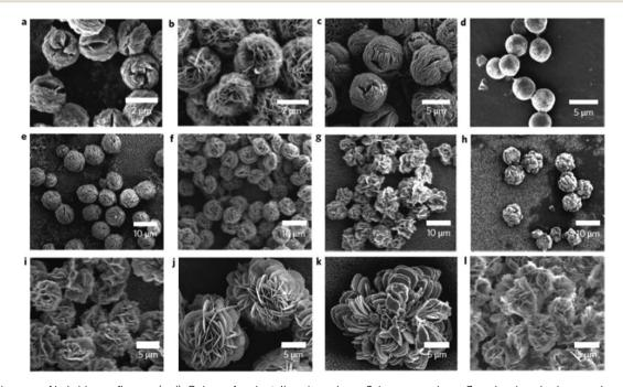
Fig. 8 SEM images of hybrid nanoflowers (a–l), Column 1,  $\alpha$ -lactalbumin; column 2, laccase; column 3, carbonic anhydrase; column 4, lipase; at protein concentrations of 0.5 mg ml<sup>-1</sup> (a–d), 0.1 mg ml<sup>-1</sup> (e–h) and 0.02 mg ml<sup>-1</sup> (i–l)<sup>108a</sup>. This figure has reproduced from ref: J. Ge, J. Lei and R. N. Zare, *Nat. Nanotechnol.*, 2012, 7, 428–43 with permission from Nature Publishing Group.
