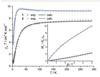
Fig. 5 Temperature dependence of  $\chi_m T$  at 0.1 Tesla for compounds 1 and 2; inset: field dependence of the molar magnetisation  $M_m$  at 2 K; circles: experimental data, solid graphs: least-squares fits.
