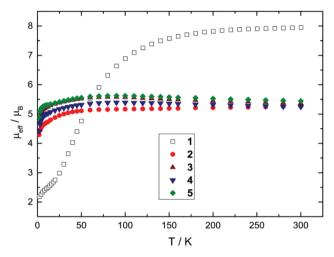
Fig. 2 Effective magnetic moment  $\mu_{\rm eff}$  vs. T plots for 1 and NHCadducts 2-5 (recorded in an applied magnetic field of 0.1 T).
