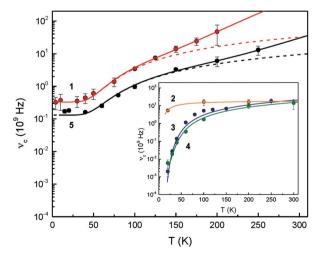
Fig. 6 Temperature-dependent relaxation rates  $\nu_c = \tau_c^{-1}$  for complexes 1-5. The broken lines consider only the spin-spin and Orbach relaxation term of ean (1) to illustrate the different contributions from Orbach and Raman type spin-lattice relaxation mechanisms. The full line represents the result of a least-squares fitting routine based on eqn (1).
