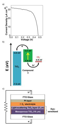
Fig. 7 (a) J-V plot for DSSCs after 3 has been adsorbed for dye-sensitization. (b) Band alignment for DSSC incorporated with 3, showing the relative energy levels (in eV against vacuum) for 3,  ${\rm TiO_2}$ , and the  ${\rm I^-/I_3^-}$  electrolyte. (c) General device structure for the DSSCs prepared in this study.
