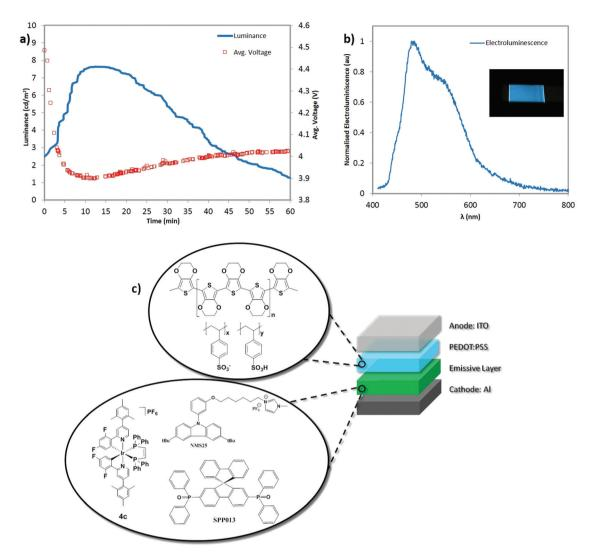
Fig. 5 (a) Luminance (solid blue line) and average voltage (open red squares) for ITO/PEDOT:PSS/active layer/Al (active layer = 1:1 by mass of NMS25: SPPO13 with 10 wt% of 4c) with a pulsed driving regime (block-wave pulsed current; 1000 Hz; 50% duty cycle; average density 100 A m<sup>-2</sup>). (b) Electroluminescence spectrum with inset photo of LEEC. (c) Schematic representation of the LEEC architecture.
