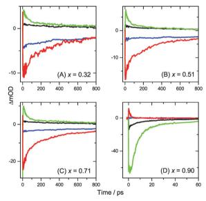
Fig. 5 Kinetic traces extracted from transient PSCP broadband absorption spectra for (MAI)<sub>x</sub>(PbI<sub>2</sub>)<sub>1-x</sub>/TiO<sub>2</sub>/glass samples. Panels (A–D) are for  $x=0.32,\,0.51,\,0.71$  and 0.90, respectively. Black and green lines are for 2 and 50 μJ cm $^{-2}$  fluence at  $\lambda_{\rm probe}=600$  nm. Blue and red lines represent 2 and 50 μJ cm $^{-2}$  fluence at  $\lambda_{\rm probe}=750$  nm.
