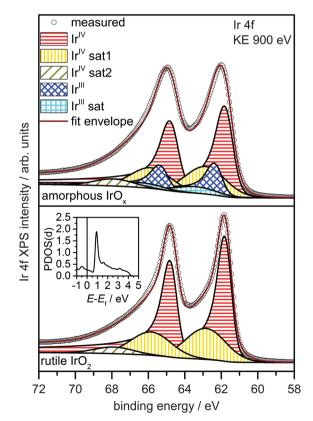
Fig. 2 Theory-based fit models for rutile IrO<sub>2</sub> (below) and amorphous  $IrO_x$  (above). The inset shows the unoccupied PDOS(d) of rutile  $IrO_2$  in presence of an Ir 4f core hole. The sharp feature  $\sim 1$  eV above  $E_f$  causes the shake-up satellite to appear at  $\sim 1$  eV above the main line.
