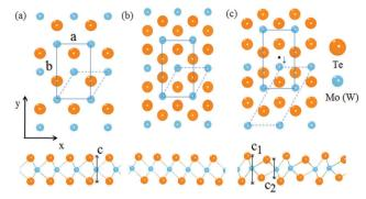
Fig. 1 Schematic representation of the structures of different phases including 2H (a), 1T (b) and 1T' (c) for MoTe<sub>2</sub> and WTe<sub>2</sub>.
