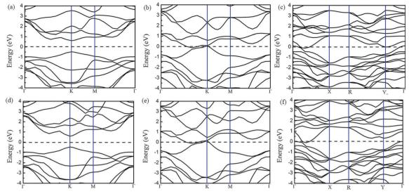
Fig. 7 Electronic band structures of monolayer MoTe<sub>2</sub> with 2H (a), 1T (b) and 1T' (c) phases and those of monolayer WTe<sub>2</sub> with 2H (d), 1T (e) and 1T' (f) phases. Note that the horizontal dashed line at 0 eV denotes the Fermi level and R presents the high symmetry k-points (0.5, 0.5 0) in the Brillouin zone.
