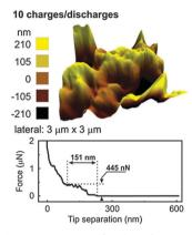
Fig. 8  $\,$  3D AFM of electrodeposited Ge after 10 charge–discharge cycles in 0.5 M LiTFSI–[Py<sub>1,4</sub>]TFSI along with the force distance curve.
