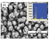
Fig. 1 (a) Cyclic voltammetry of 0.25 M GeCl<sub>4</sub>-[Py<sub>1.4</sub>]TFSI on Cu. The scan rate was 10 mV s<sup>-1</sup>, (b) the morphology of the electrodeposited Ge at constant potential of -1.9 V for 30 minutes, the inset shows the EDX of the electrodeposit.
