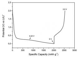
Fig. 4 First charge-discharge cycle of 0.5 M LiTFSI-[Py<sub>1.4</sub>]TFSI on electrodeposited Ge on Cu. The current density was 200  $\mu\text{A}~\text{cm}^{-2}$  during both charge-discharge processes. The arrows marked are the cut-off voltages used for investigating the SEI layer formation.
