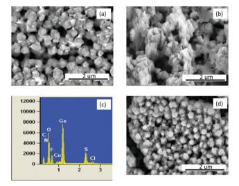
Fig. 5 (a) Microstructure obtained after charging the electrodeposited Ge until a cut-off voltage of 0.22 V (b) complete charge of the electrodeposited Ge until a cut-off voltage of 0 V (c) EDX of (b) and (d) one charge-discharge cycle until a cut-off voltage of 2.0 V.
