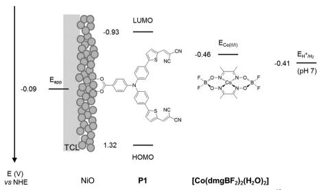
Fig. 2 Energy diagram of NiO-P1-[Co(dmgBF<sub>2</sub>)<sub>2</sub>(H<sub>2</sub>O)<sub>2</sub>] electrodes (note: potentials of P1 in MeCN from Qin et al. <sup>16</sup> and for [Co(dmgBF<sub>2</sub>)<sub>2</sub>(H<sub>2</sub>O)<sub>2</sub>] in pH 7 phosphate buffer corrected vs. NHE from Berben et al. <sup>20</sup>). TCL: transparent conducting layer.
