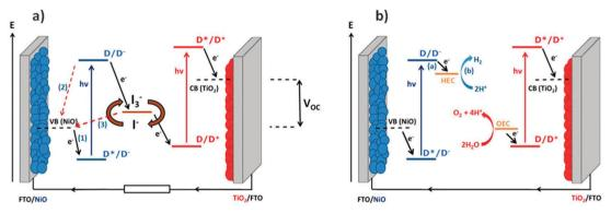
Fig. 1 Schematic illustration of (a) a tandem dye-sensitized solar cell and (b) a dye-sensitized photoelectrosynthetic cell. (VB: valence band; CB: conduction band; HEC: hydrogen evolution catalyst; OEC: oxygen evolution catalyst).
