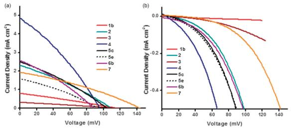
Plot of current density vs. voltage curves (a) under AM1.5 illumination and (b) in the dark for the NiO DSCs.
