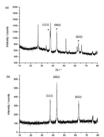
**Fig. 5** Representative X-ray diffraction patterns for sample **4**: (a) the NiO film on FTO; (b) the NiO nanoparticles removed from the film. The diffraction peaks indexed with the (*hkl*) notation correspond to the main NiO phase.<sup>25</sup> \* Denotes the peaks corresponding to NiO.
