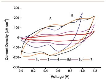
Fig. 7 Cyclic voltammograms of the different NiO preparations, recorded in phosphate buffer (0.05 M pH 7) at a scan rate of 20 mV s<sup>-1</sup>.
