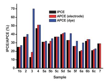
Fig. 8 Summary of all IPCE measurements and the derived APCE at 500 nm. The filled (first) bar indicates the IPCE value, the red bar (second) indicates the APCE calculated from the absorption spectrum of the complete electrode, and the blue (third) shows the APCE calculated from the difference dye spectrum of the surface
