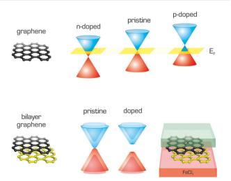
Fig. 8 Band structure of single layer graphene showing p- and n-type doping with respect to the Fermi level, and band gap opening in bilayer graphene caused by doping
