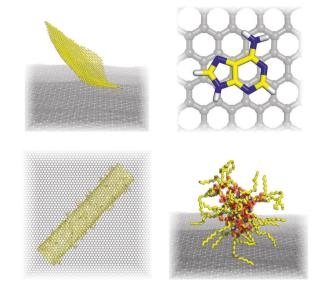
Fig. 7 Screenshots from molecular dynamics simulations of various processes taking place on a graphene surface: graphene exfoliation (top left), nucleobase adsorption (top right), graphene···carbon nanotube assembly (bottom left), and the formation of a reverse lecithin micelle on a graphene surface.
