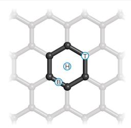
On bond (B), top (T), and hollow (H) adsorption sites on graphene.
