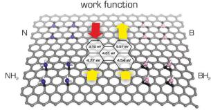
Fig. 6 The work functions ( $W_f$ s) calculated using the PBEO functional of B/N-doped graphenes vary with the chemical nature of doping.  $^{162}$  The  $W_f$ value of pristine graphene 4.31 eV (shown in the middle) increases in substitutionally B-doped graphene to 5.57 eV and decreases to 3.10 eV in substitutionally N-doped graphene. On the other hand, the  $W_f$  values increase in both graphenes with added  $-NH_2$  and  $-BH_2$  groups to 4.77 and 4.54 eV, respectively.
