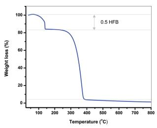
Fig. 5 The thermogravimetric diagram of  $6\cdot 0.5C_6F_6$  showing the loss of the  $C_6F_6$  solvate at 140 °C and the decomposition of  $\bf 6$  at 280 °C.
