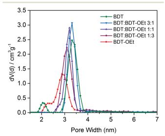
**Fig. 4** Detail of the pore size distributions of BDT COF, mixed BDT: BDT-OEt COFs and BDT-OEt COF showing the decrease of the main pore diameter upon the incorporation of ethoxy side chains into the COF structure.
