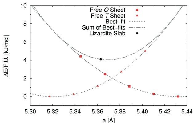
Fig. 2 Strain energy per formula unit of free-standing flat T and O sheets [ $\text{kJ mol}^{-1}$ ] as a function of the unit cell parameter [ $\text{\AA}$ ]. The superimposed dotted curves have been obtained through quadratic best-fit over the corresponding datasets; the dash-dotted curve is the sum of the former two. Also shown for sake of comparison is the value of the cell parameter for the flat lizardite slab (its position along the y axis is arbitrary).
