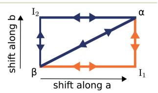
Fig. 2 A schematic overview of the three possible routes, direct and along a and b, that lead to a transition from the  $\beta$  to the  $\alpha$ . The most likely route as obtained from an earlier study<sup>14</sup> is depicted in orange.
