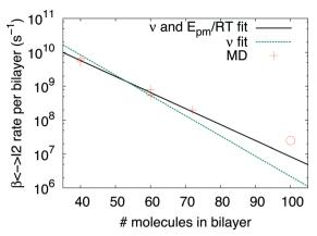
Fig. 5  $\beta \mapsto I_2$  shifting rate obtained from MD simulations<sup>14</sup> with different simulation cell sizes as a function of number of molecules in a bilayer. The solid and dashed lines are results of fits of eqn (2) to the data crosses (see text for details). The circle is based on a single transition.
