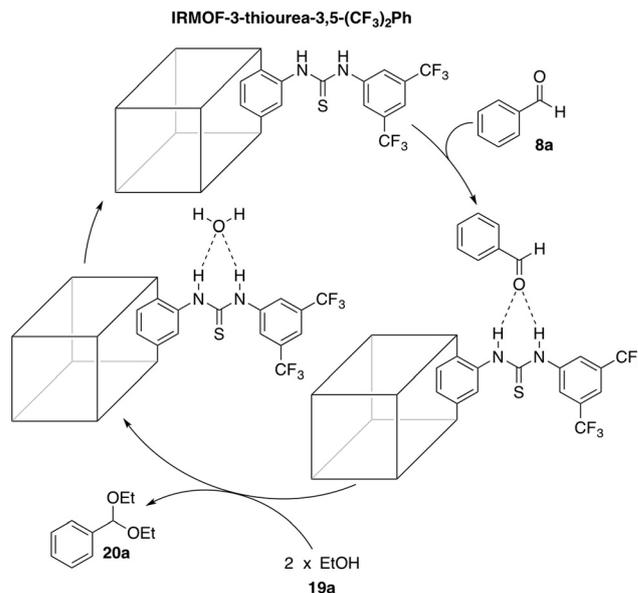
**Scheme 8** Mechanistic proposal for the acetalisation reaction catalysed by **IRMOF-3-thiourea-3,5-(CF<sub>3</sub>)<sub>2</sub>Ph**.<sup>56</sup>
