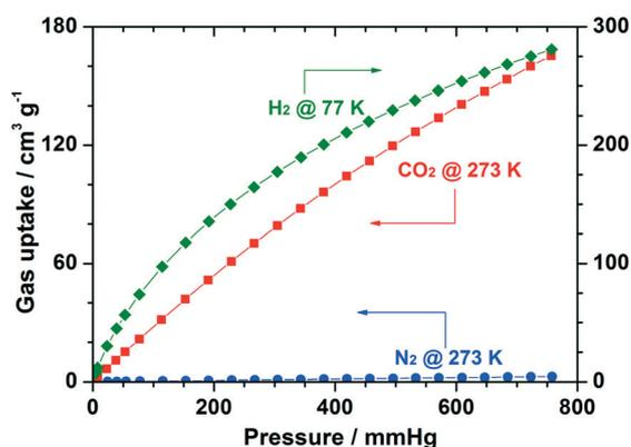
**Fig. 7** Gas sorption isotherms of Cu-UBTA for CO<sub>2</sub> and N<sub>2</sub> (at 273 K), and H<sub>2</sub> (at 77 K). Reprinted with permission from ref. 55. Copyright © Royal Society of Chemistry.
