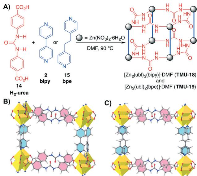
**Scheme 5** A) Synthesis of catalytic urea-containing MOFs TMU-18 (trigonal *P*<sub>1</sub>) and TMU-19 (orthorhombic *Pnna*). B) and C) View along the pore direction of TMU-18 and TMU-19, respectively. In contrast to TMU-18, TGA analysis indicated a lower thermal stability for TMU-19. Adapted with permission from ref. 53. Copyright © Royal Society of Chemistry.
