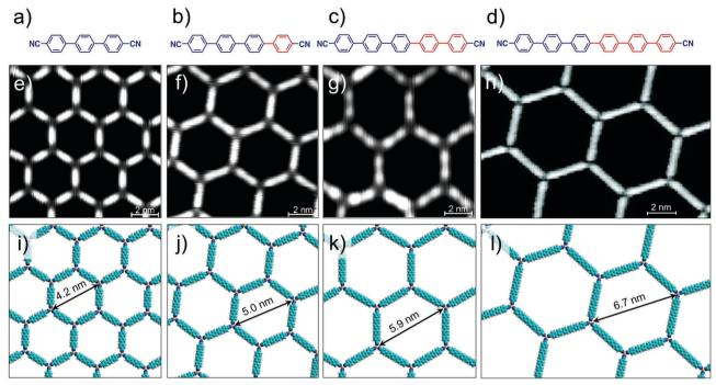
Fig. 4 Isoreticular host networks based on metal-ligand coordination. (a-d) Molecular structures of dicarbonitrile-polyphenylene (NC-Ph<sub>n</sub>-CN) building blocks with increasing the length of the oligophenylene backbone. Corresponding STM images of the host networks for (e) n = 3 (f) n = 4(q) n = 5 and (h) n = 6. Panels (i–l) show molecular models for the corresponding porous networks, respectively. Reproduced from ref. 58 and 59 with permission from the American Chemical Society
